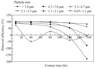
Fig. 5 Removal efficiencies of particles in each size.
