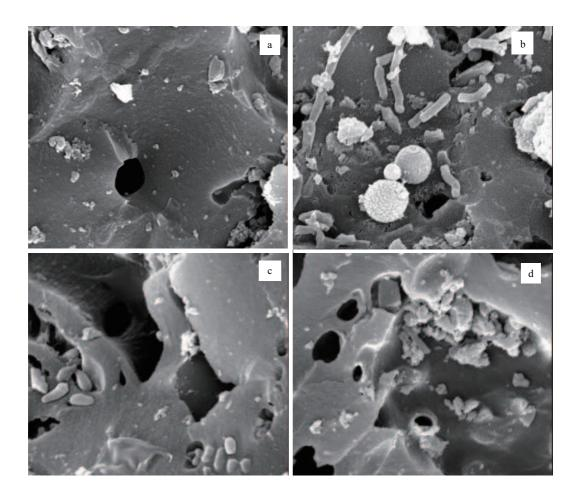
Fig. 10 SEM of the activated carbon (×10,000). (a) new activated carbon; (b) used activated carbon; (c) regenerated by UV; (d) regenerated by high pressure vapor.
