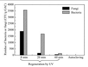
Fig. 9 Residue of bacteria and fungi on the activated carbon after regeneration.
