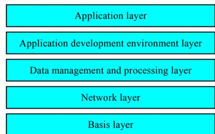
Fig.4 Abstract structure of sensor networks
