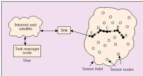
Fig.2 Structure of a typical sensor network
